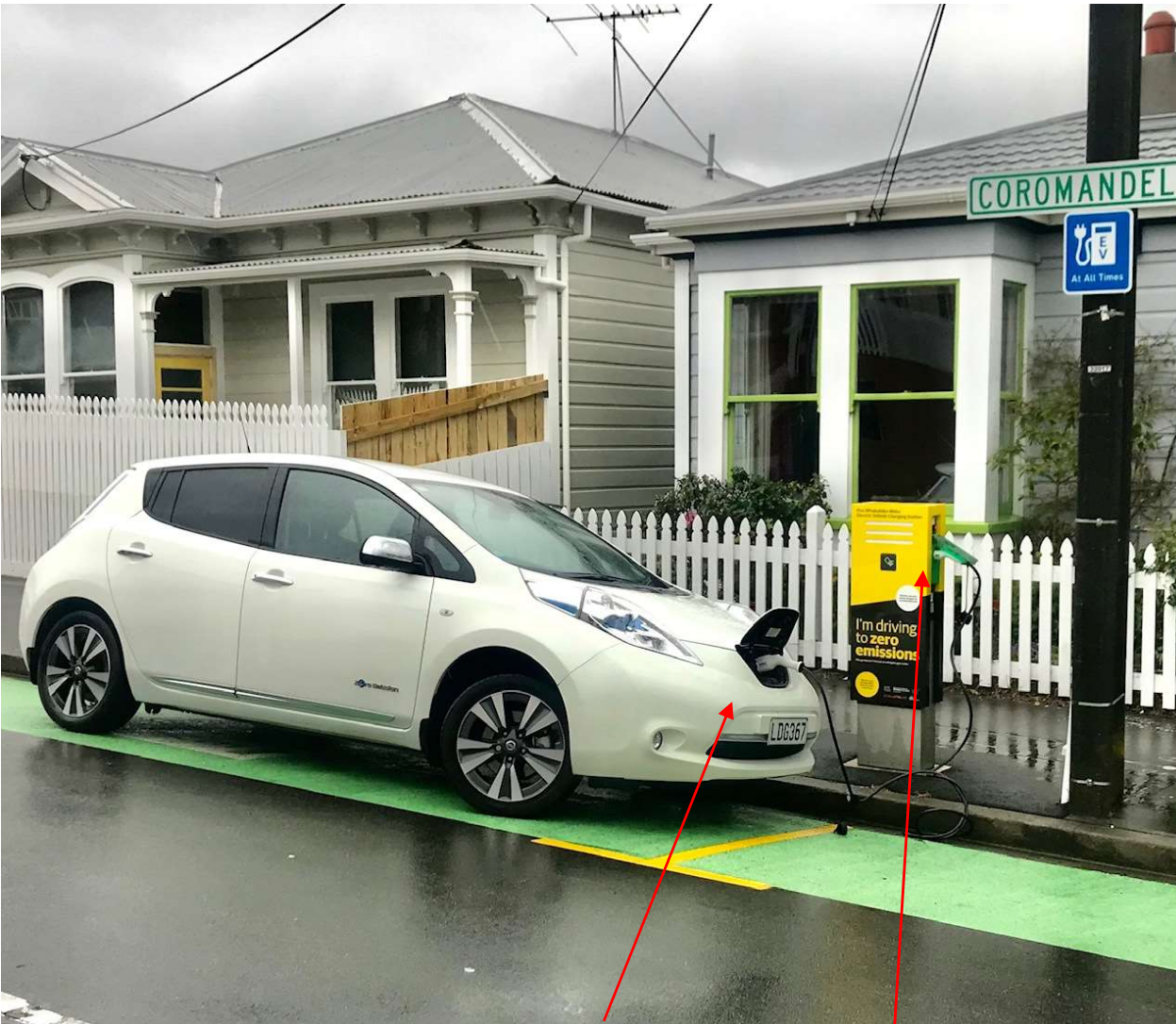
Portable cable with: Type 1 at EV and Type 2 at charger
