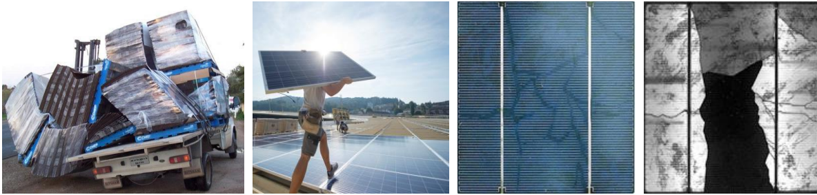
Appearance of "SNAIL TRAILS" (big jerks during transport or installer who stepped on it)
